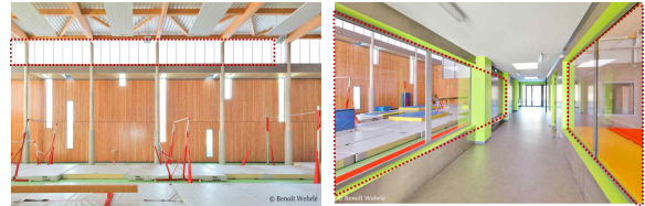
Figure 10. Skylight for privacy & corridors for watching training area
